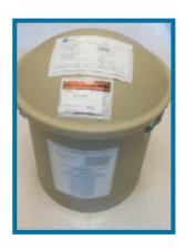
Cryogenic vessel does NOT contain liquid nitrogen, only vapor is present inside shipper, therefore, a vapor fog will be present when opening vessel.
