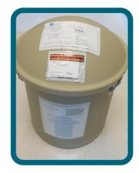
3) Cryogenic vessel does NOT contain liquid nitrogen, only vapor is present inside shipper, therefore, a vapor fog will be present when opening vessel.
